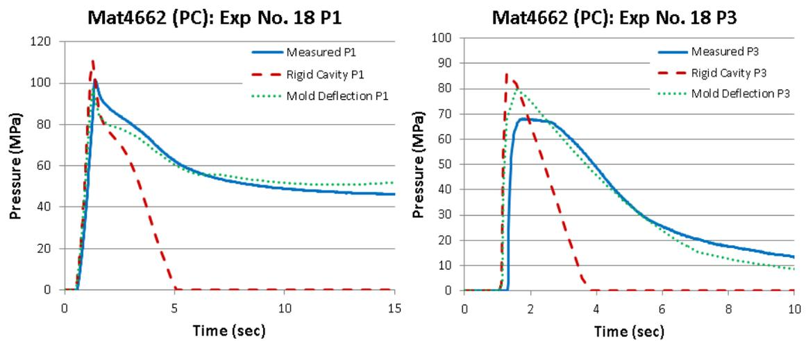
Figure 6 – Cavity pressure traces for Mat4662 Molding Experiment Number 18
