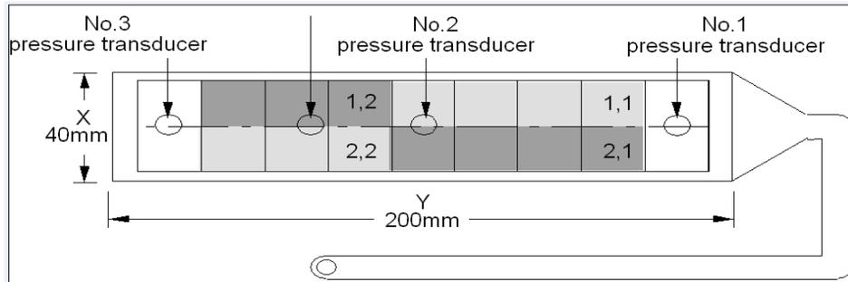
**Figure 1** – Geometry of instrumented mold
