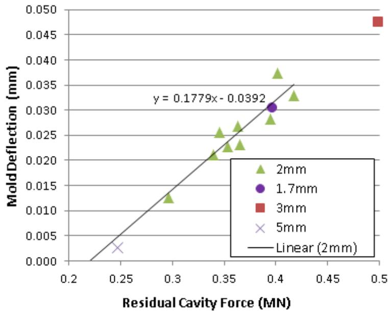
Figure 2 – Mold deflection characteristic for a PC+ABS dataset
