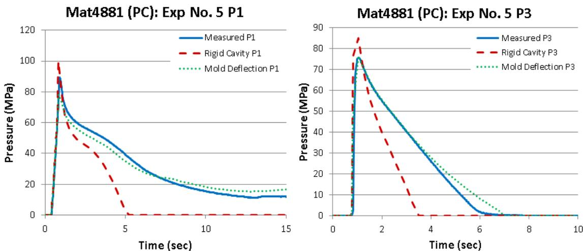
Figure 8 – Cavity pressure traces for Mat4881 Molding Experiment No. 5
