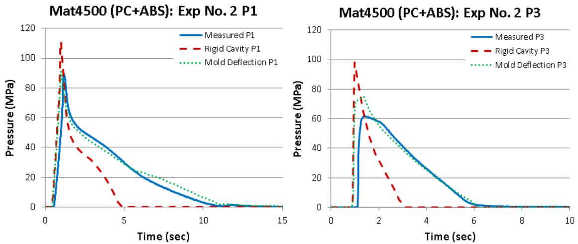
Figure 5 – Cavity pressure traces for Mat4500 Molding Experiment Number 2
