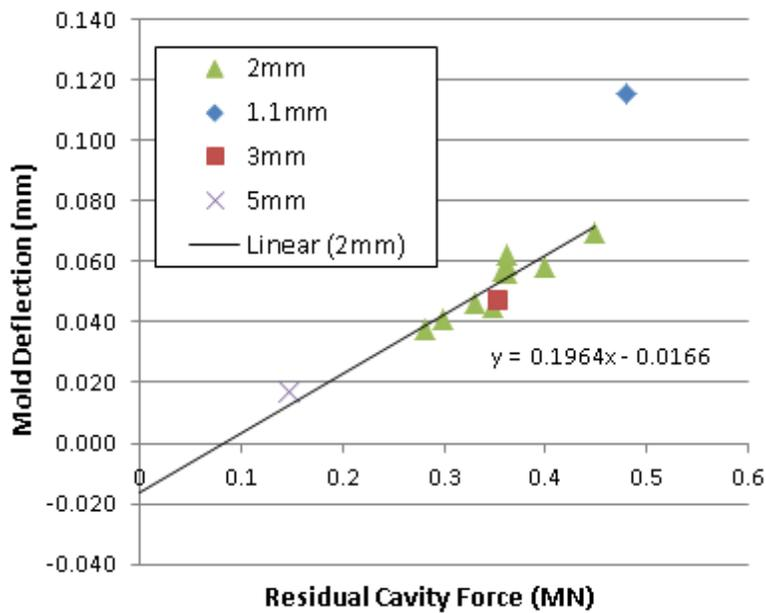
Figure 3 – Mold deflection characteristic for a PET dataset
