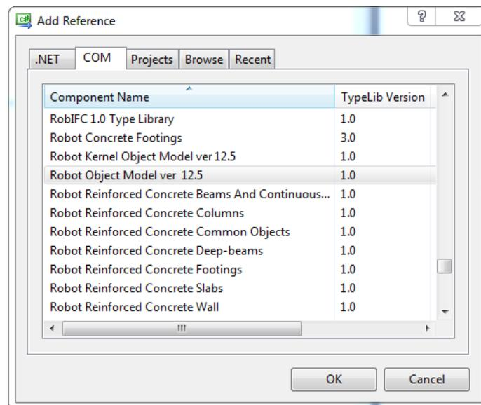
Then you need to write using Robot OM; in the top of your program file:
