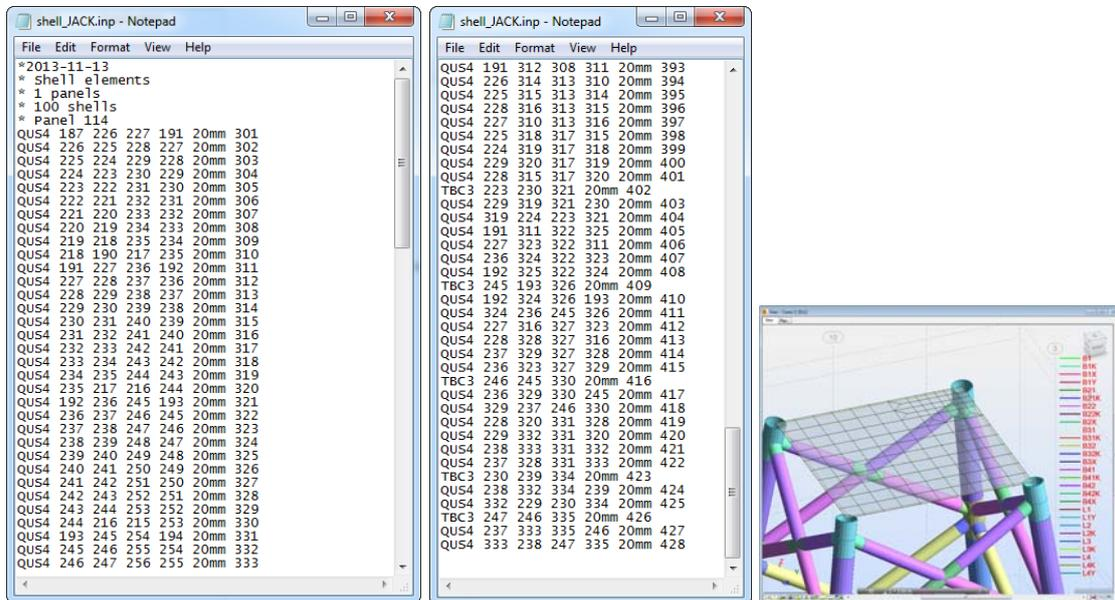
Here the program can write out both 3 noded or 4 noded shell elements with the appropriate definition for ANSYS ASAS.
