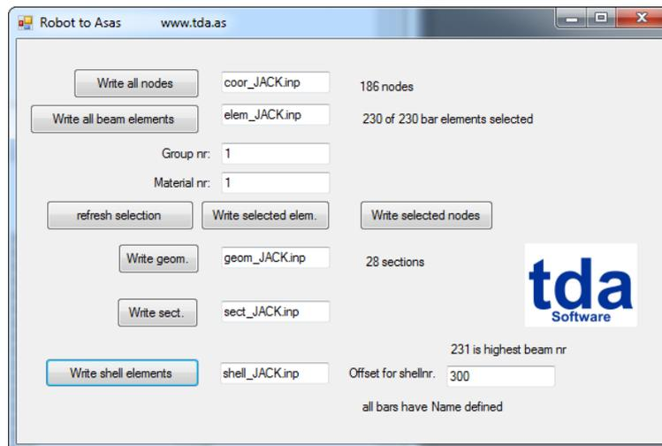
The format of the files is that one line typically defines an element and text after the \* is a comment, therefore ignored by ANSYS ASAS. The first file is the node file which includes the node number, and coordinates in x, y and z.
