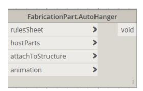
The hanger placement tool consumes the "FabricationPart.AutoHanger" block, in the graph shown as below:
