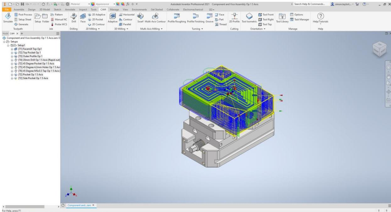
We can apply machining strategies on a 3D Model and then run a simulation to ensure it is giving us the results we would expect, see below: -
