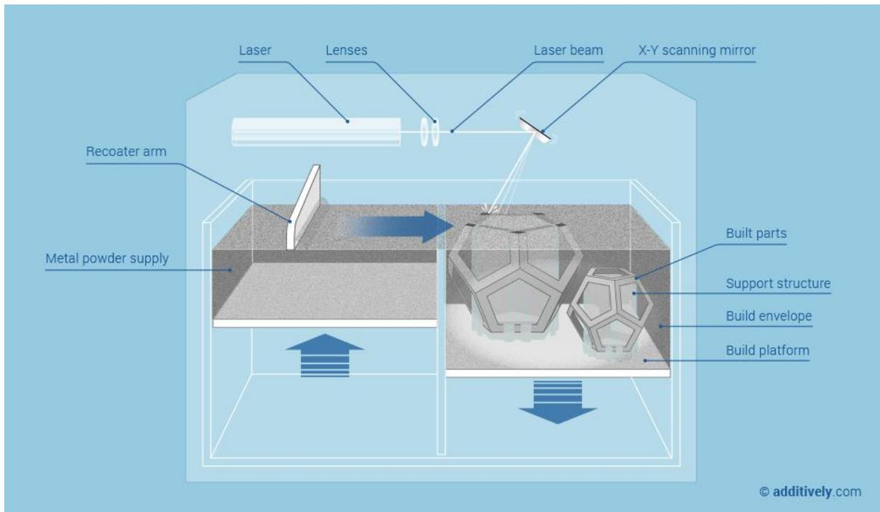
FIGURE 2: WHAT IS LASER POWDERBED FUSION? (SOURCE: ADDITIVELY).
