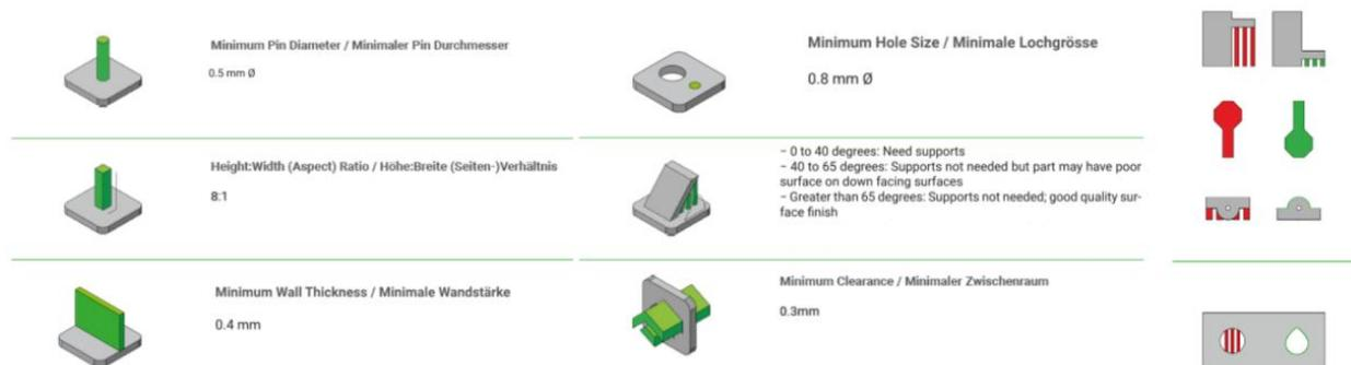
FIGURE 9: DESIGN GUIDE RULES (SOURCE: ONE CLICK METAL).
