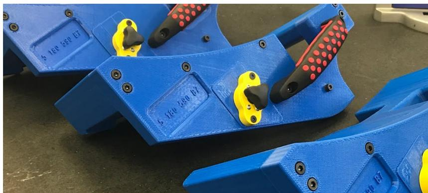
*FDM JIGS USED IN VEHICLE ASSEMBLY OPERATIONS MADE WITH BLUE ABS*
