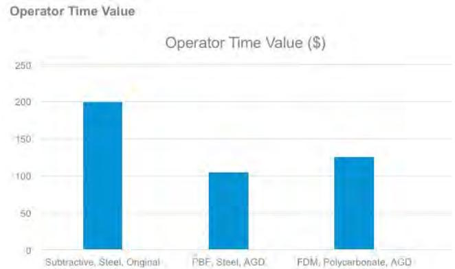
Fig. 8: Operator time value per process. Simplified AM processes lead to decreased hands on operator costs.
