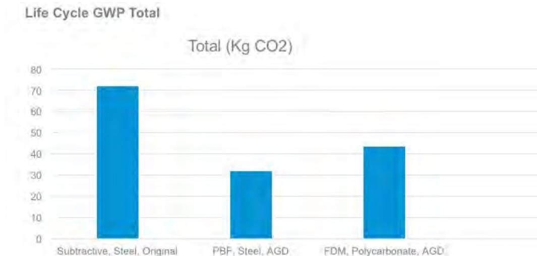
Fig. 4: The total life-cycle Global Warming Potential in KgCO2 for each part and process.
