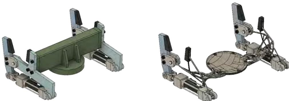
Fig.1: The original end-effector part (left) and the generatively designed part (right) in context.
