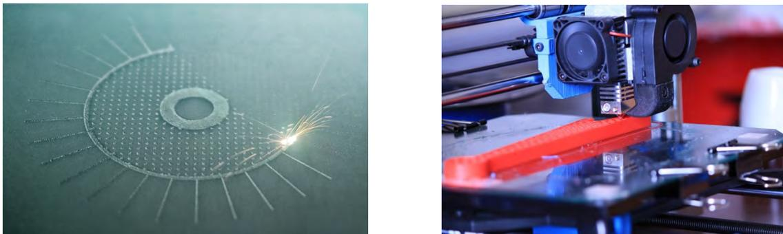
Fig 2: Powder Bed Fusion (PBF) and Fused Deposition Modeling (FDM) technologies
