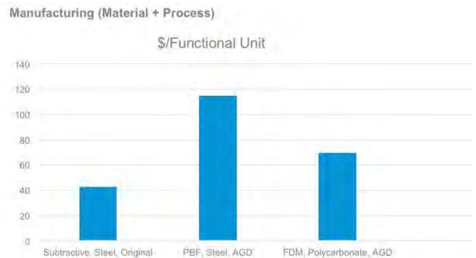
Fig. 7: Primary manufacturing costs including processed input material and machine electricity costs.
