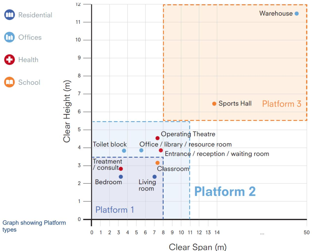
The Platform system saves effort throughout the entire process – the design, manufacturing, delivery and assembly. Design effort should be spent where it can add the most value – creating places that people want to live and work. This standard kit of parts can be configured to offer a broad range of building products without limiting design ambition. If a design idea cannot be achieved with the current platform system, then the parts list is expanded.
