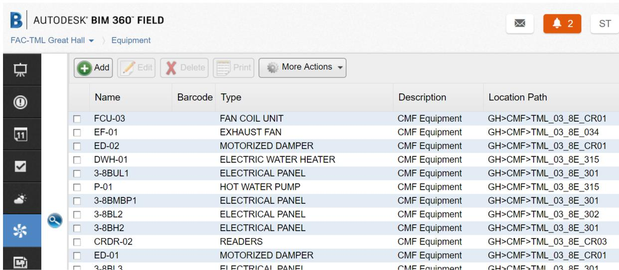
The screenshot shows the Autodesk BIM 360 Field interface. At the top, it displays 'AUTODESK BIM 360 FIELD' and 'FAC-TML Great Hall > Equipment'. Below the header is a toolbar with 'Add', 'Edit', 'Delete', 'Print', and 'More Actions' buttons. The main area contains a table of equipment assets.
