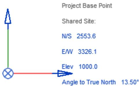
**Project Base Point:** Autodesk explains “The project base point can be used to establish a reference for measuring distances and positioning objects in relation to the model.” It can be used for aligning models being linked into one another and for controlling setting out from a local point on-site. As of Revit 2020, when you move the point, it no longer modifies the Shared Coordinate grid however typing into the Angle to True North still modifies the project.
