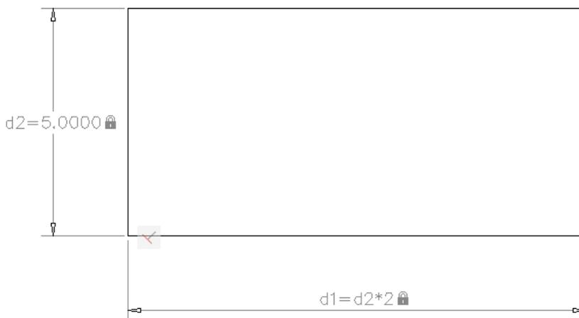
The example above contains a rectangle with two dimensional constraints where the length ( $d1$ ) is equal to twice the height ( $d2$ ).
