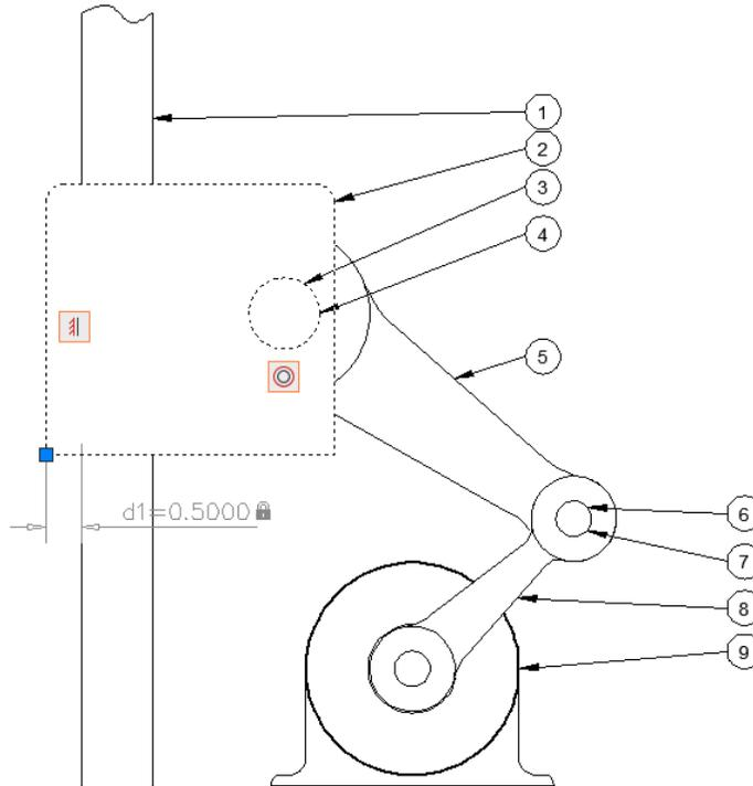
2. Select the block representing the slider on the shaft (identified by callout number 2).
