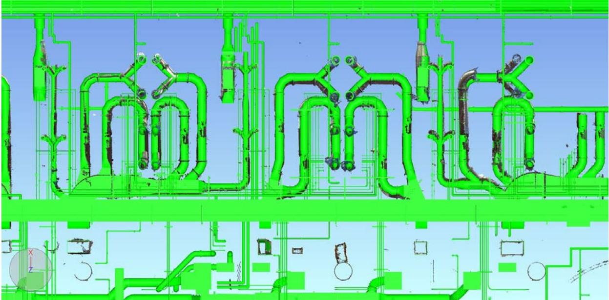
Mid-Construction scanning involves leveraging the technology to validate 'planned vs installed work'. This can be helpful to quickly ensure the scope in a Building Information Model has been installed as coordinated, check for stub-up/rebar/PT prior to a slab pour, ensure walls are plumb and verify floor flatness, and track structural settlement/deflection over time. Our Mid-Construction scanning process has come to be known as 'Construction Verification.'
