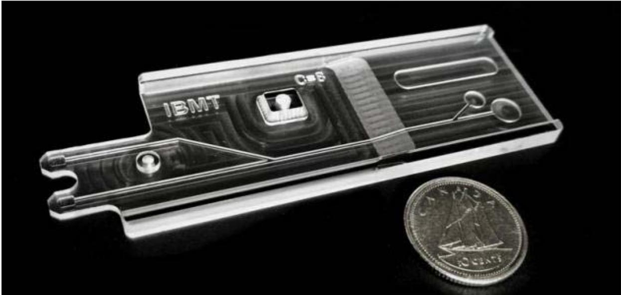
FIGURE 3: A MICROFLUIDIC DEVICE MACHINED ON TORMACH PCNC 770. PHOTO CREDIT: EDMOND YOUNG, UNIVERSITY OF TORONTO
