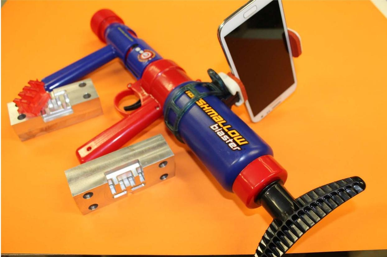
FIGURE 4: WITH A COMBINATION OF SHORT-RUN CNC MACHINED INJECTION MOLDS AND MACHINED RIGID PLASTIC PARTS, MARSHMALLOW FUN CLUB WAS ABLE TEST MARKET THEIR “MARSHMALLOW BLASTER” AT THE NY TOY FAIR BEFORE ORDERING EXPENSIVE PRODUCTION TOOLING FOR MASS PRODUCTION
