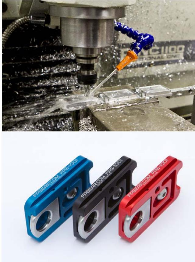
FIGURE 8: THE LONG PARALLEL EDGES OF THIS CAMERA ADAPTOR IS A NATURAL FIT FOR A “FLIP AND DECK” WORKHOLDING STRATEGY USING A MACHINIST VICE.
