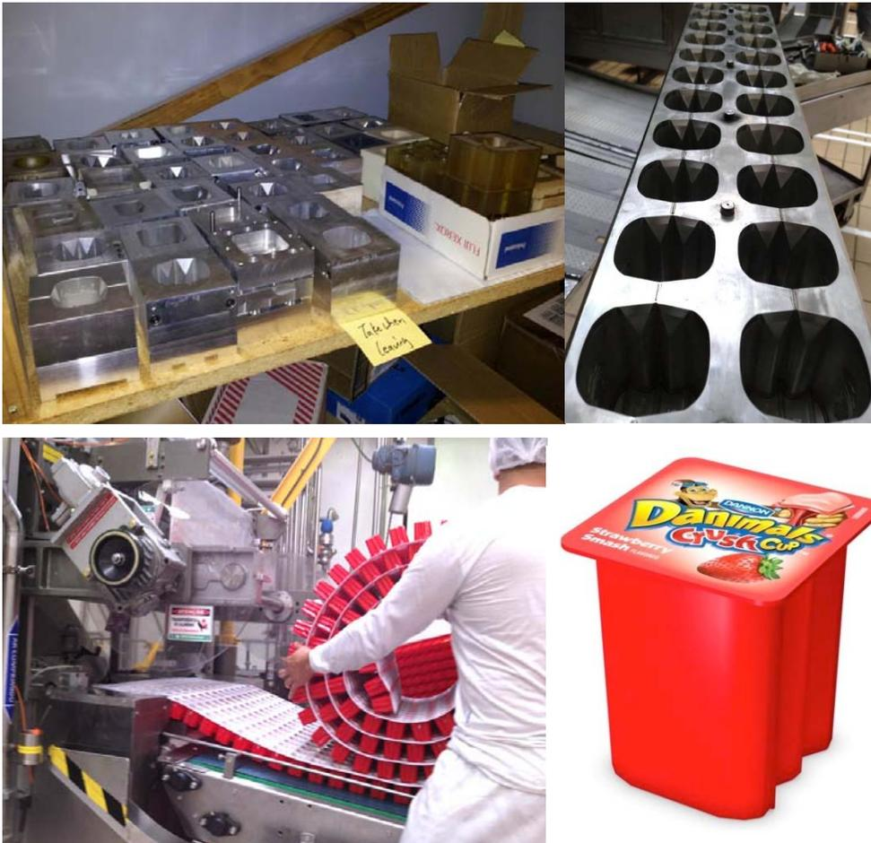
FIGURE 5: PRODUCT DESIGNER EDWARD SCOTT CREATED OVER 25 DIFFERENT PROTOTYPE MOLDS USING A TORMACH PCNC 1100 TO PROVE OUT HIS CONCEPT FOR THE “CRUSH CUP” BEFORE INVESTING IN PRODUCTION TOOLING.
