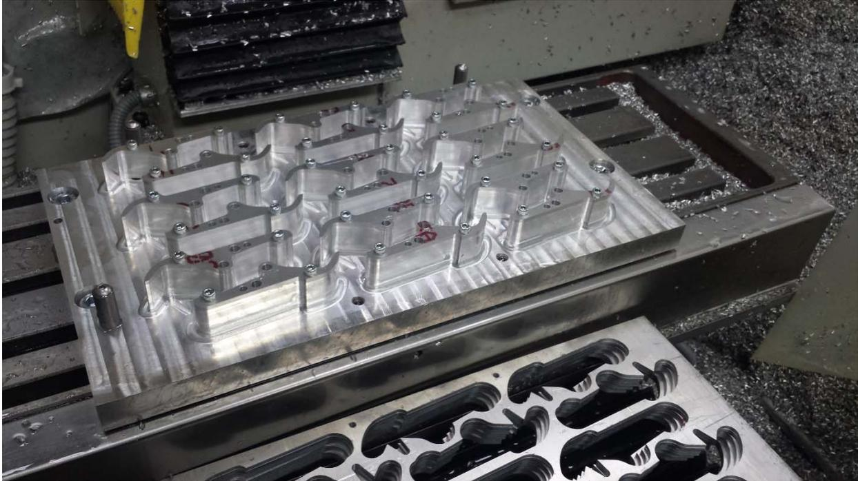
FIGURE 9: THESE PARTS ARE MACHINED BY FIRST USING A "PICTURE FRAME" WORKHOLDING TECHNIQUE TO ROUGH MILL THE PERIMETER PROFILE BEFORE A SECOND FINISHING MILLING OPERATION ON A FIXTURE PLATE.
