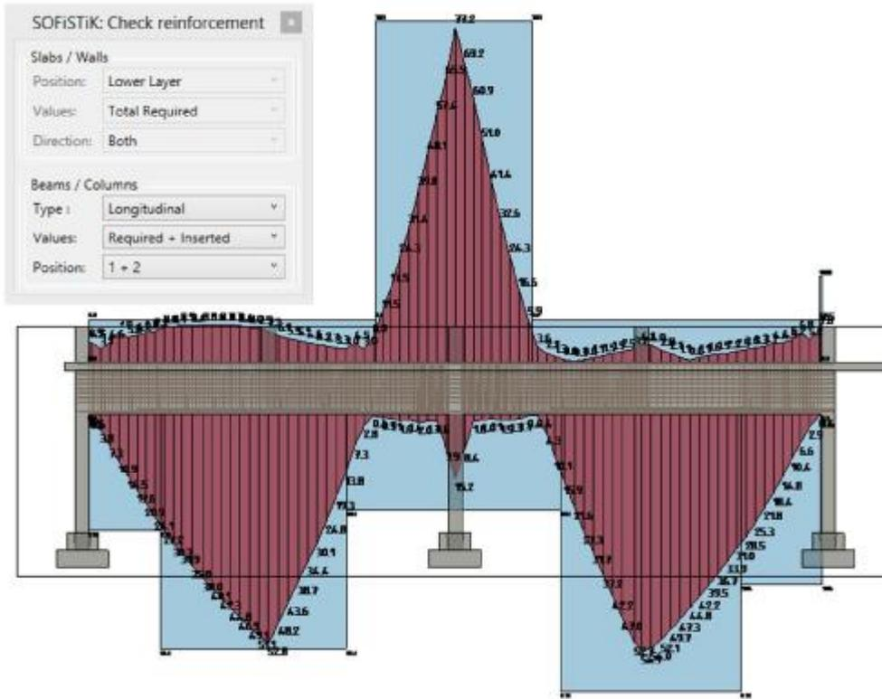
For beams and slabs a presentation as areas is common and well arranged. For slabs a presentation as scaled crosses has the advantage, that values of two directions and the angle of the reinforcement can be displayed in a single view.
