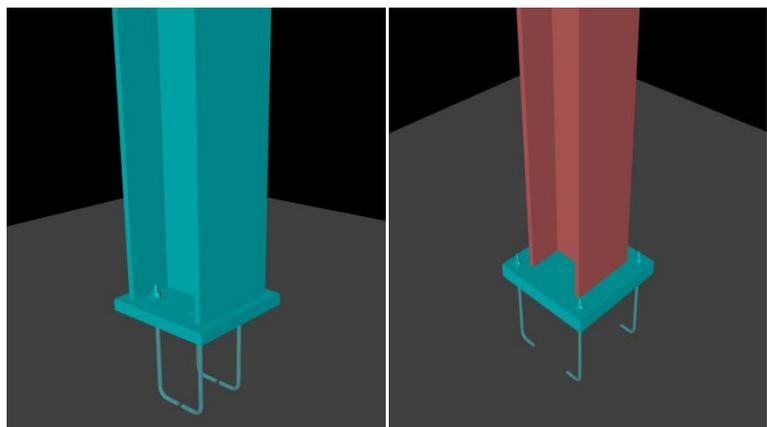
base plates are required to be oversized (anchor bolts outside of footprint and/or require a recessed pocket in the slab to avoid tripping hazard or minimize furring area requirement around the column) or if the anchors can satisfy the design loads by staying within the confines of the column footprint. Determine the pros and cons to help guide the decision. This will help the foundation detailing as it will be identified early.
